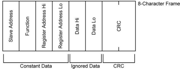
**Figure 9: Modbus RTU Preset Single Register Response**
