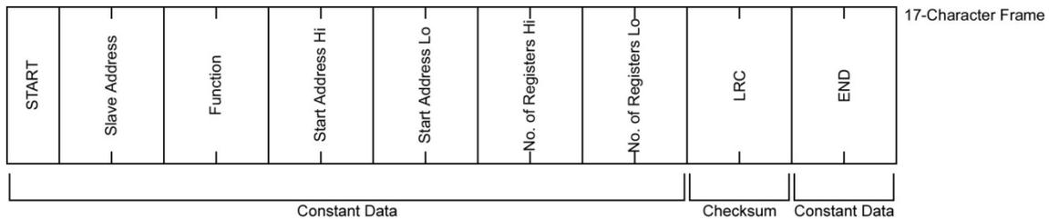
**Figure 1: Modbus ASCII Read Holding Register Request**
