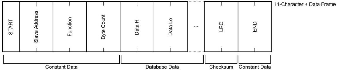
**Figure 4: Modbus ASCII Read Holding Register Response**
