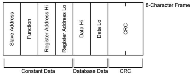
**Figure 7: Modbus RTU Preset Single Register Request**
