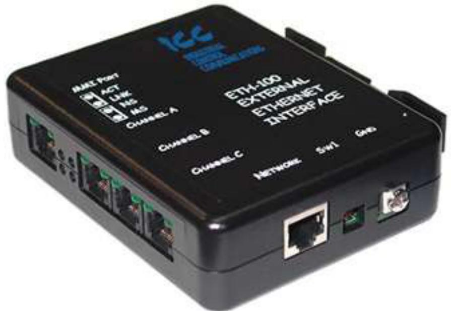
The ETH-100 provides ethernet connectivity to up to three Toshiba 7-series, 9-series or VF-nC1 Adjustable Speed Drives (ASDs) with Modbus TCP/IP, release 1.0 (Conformance class 0 and partial class 1 and class 2 compliant).
